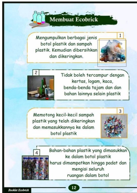
Gambar 4. 4 Bagian membuat *ecobrick*
